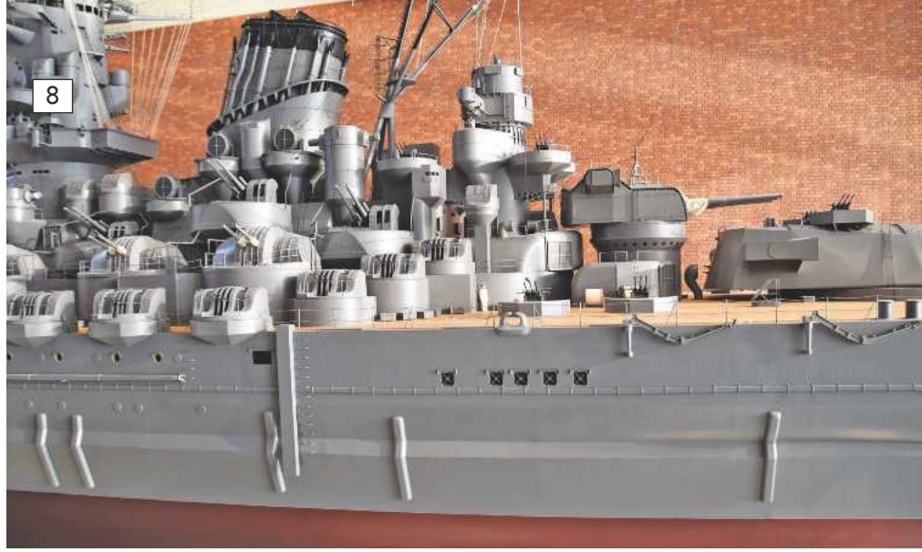
8: When completed in December 1941 a 15.5cm gun turret was positioned on the main deck level on either beam amidships.
