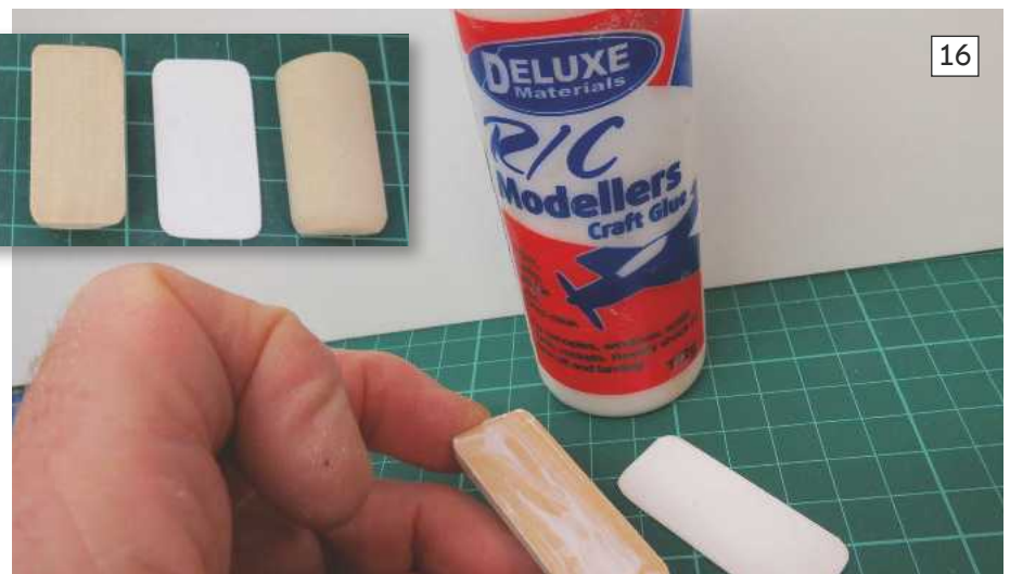
16: Using R/C modellers' glue, the two timber halves are fixed to the styrene centre profile.
