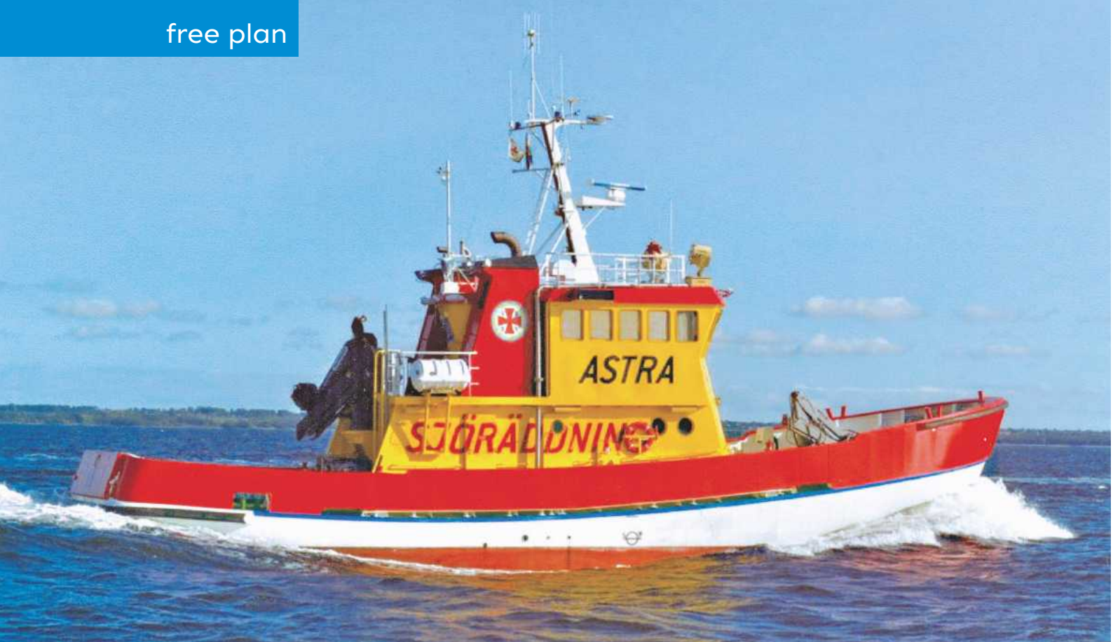
Starboard side of Astra underway. This gives a good view of colour scheme, rubber fendering at the bow and stern. Note the lettering on sides differ from that on the plan, but either will be applicable.
