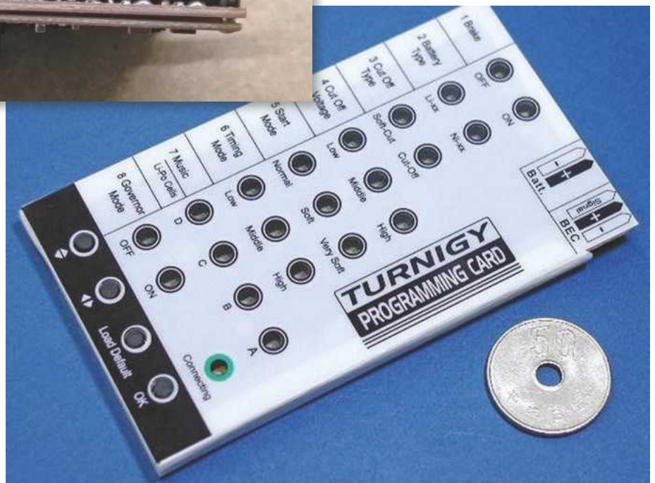
A composite picture showing a typical programming card and the USB Linker.
