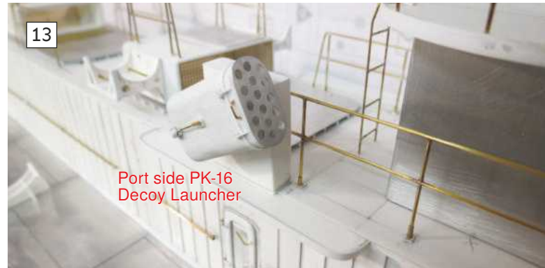
12: On the underside of the mounting two locating pins are added to ensure a firm and precise fit. 13: Port PK-16 decoy launcher in place. 14: The starboard PK-16 launcher.
