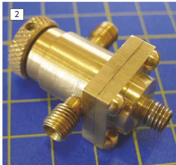
2: A purely mechanical attenuator valve as supplied by Forest Classics. The steam line is attached to the bottom connection and the gas flows through the other two ports on the body. The pressure is set by the knurled knob on the top of the valve.
