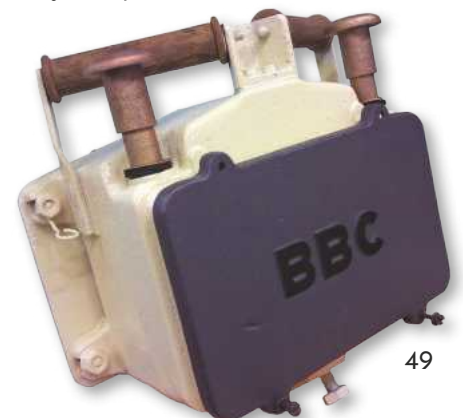
BELOW: The fully restored BBC (Dive and trim) remote guidance system.
