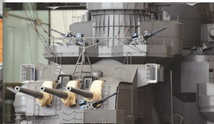
7: In 'X' position is the after 15.5cm/60calibre triple secondary armament.
