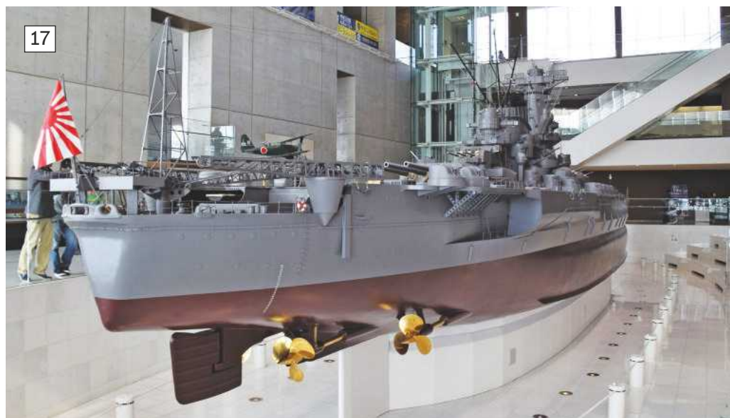
17: The final picture of this series on the battleship Yamato provides a good perspective viewing forward on the starboard side giving a full view of the rudder and shaft arrangement.
