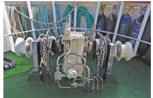
ABOVE: The forward windlass and detail of bulwark stanchions.
