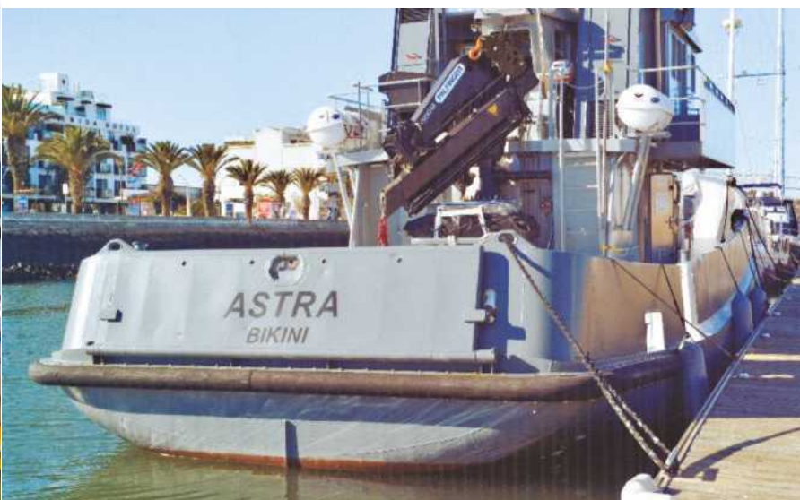
BELOW LEFT: View of the transom and hinged door and protective rubber belting. The ladder from deck to deckhouse top and life raft canisters launching cradles. This was taken in warmer climes after she was converted to a motor yacht. BELOW RIGHT: View under the stern showing detail of rudder with protective ice knife above, note protective fins on the hull ahead of the propeller, also the line of the bulb where it meets the hull plating.
