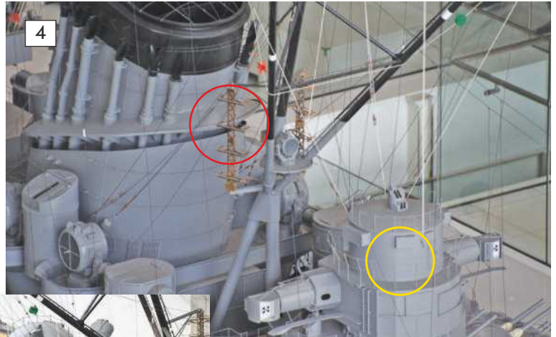
5: All of the AA outfit fitted in later years, especially those close too or on the main deck, where enclosed to protect against the blast of the 18in guns.
