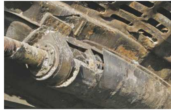
ABOVE: Depth charge damage on the starboard side.
