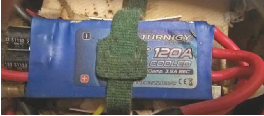
LEFT: The Turnigy Aquastar in my 4Cell Cat. Not fully waterproof, but pretty water resistant. Three Years of hard racing and still going strong. Fully programmable using a Turnigy USB Linker.
