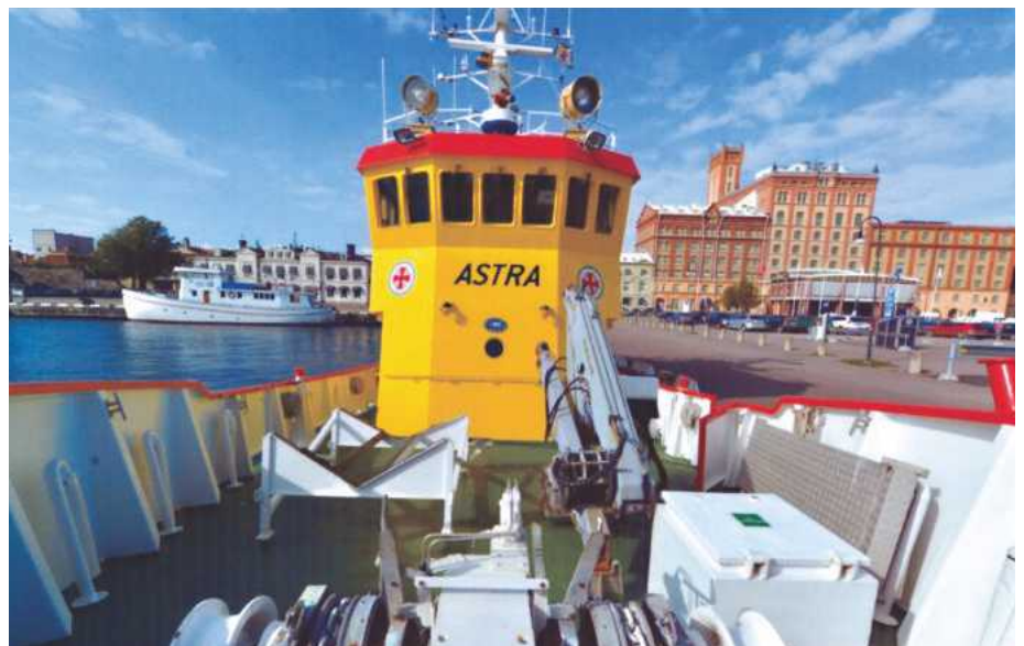
View look on front of deckhouse. Four of the wheelhouse windows have wipers fitted. Note slight overhang of wheelhouse over the lower deckhouse. Cradle for RIB and deck crane and small square hatch in the foreground.
