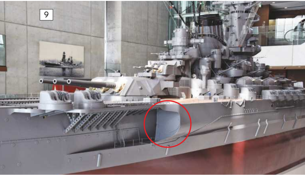
9: This starboard side aft shot shows the blast door for access into the boat stowage gallery.
