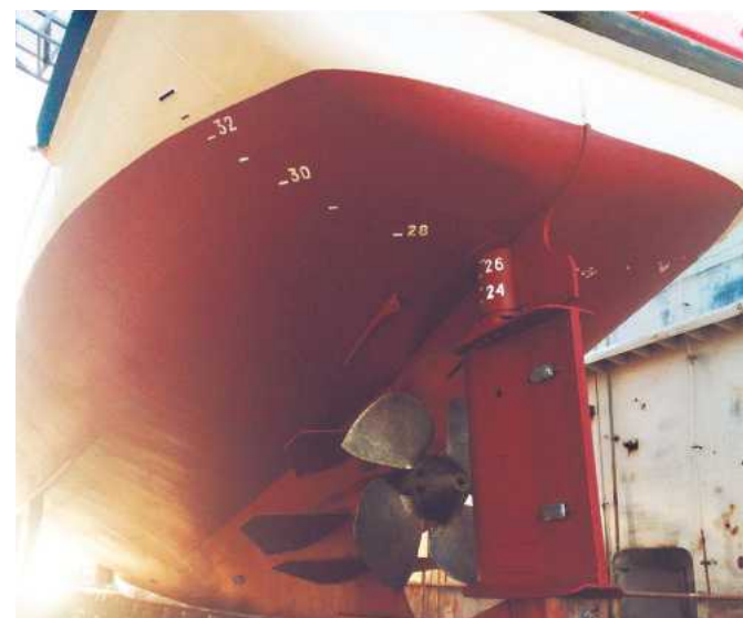
BELOW LEFT: View of the transom and hinged door and protective rubber belting. The ladder from deck to deckhouse top and life raft canisters launching cradles. This was taken in warmer climes after she was converted to a motor yacht. BELOW RIGHT: View under the stern showing detail of rudder with protective ice knife above, note protective fins on the hull ahead of the propeller, also the line of the bulb where it meets the hull plating.
