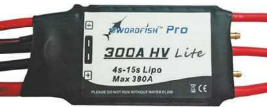
ABOVE: A 300amp Swordfish ESC which can also use the USB Linker for programming.
