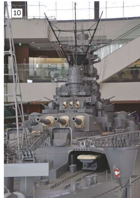
10: Here the model shows the location of the boat stowage gallery which allows the ships boats to be tracked right aft and lifted over the side.
