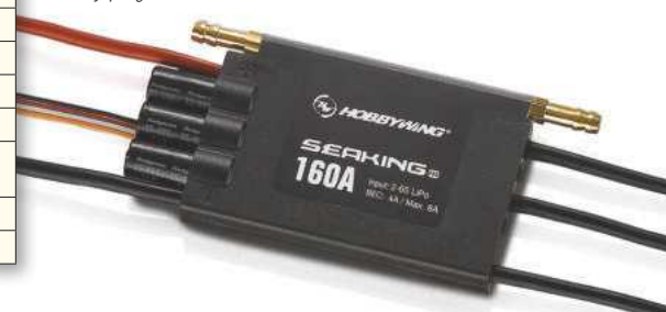
BELOW: A more normal range ESC, fully waterproof and fully programmable.
