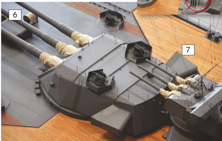
6: The total all up weight of each one of the 46cm or 18in gun turrets was a colossal, 2774tons. The AA round as fired from the 46cm guns on Yamato's last sortie could disperse 900 incendiary tubes which were ignited into the path of any incoming aircraft
