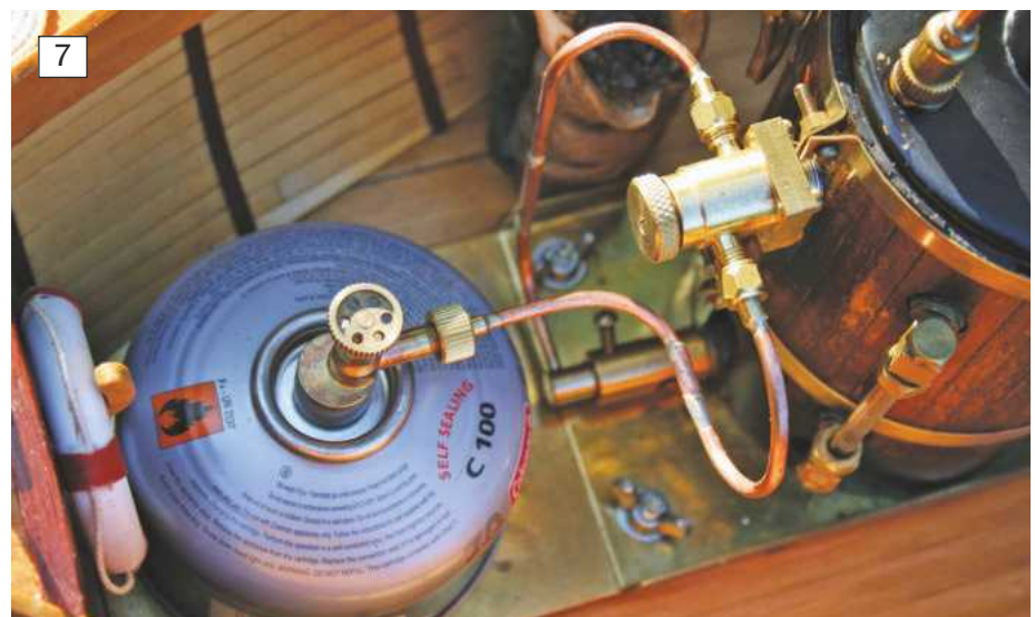
7: The boiler mounted attenuator with the disposable gas tank, mounted on a common brass base with the boiler.
